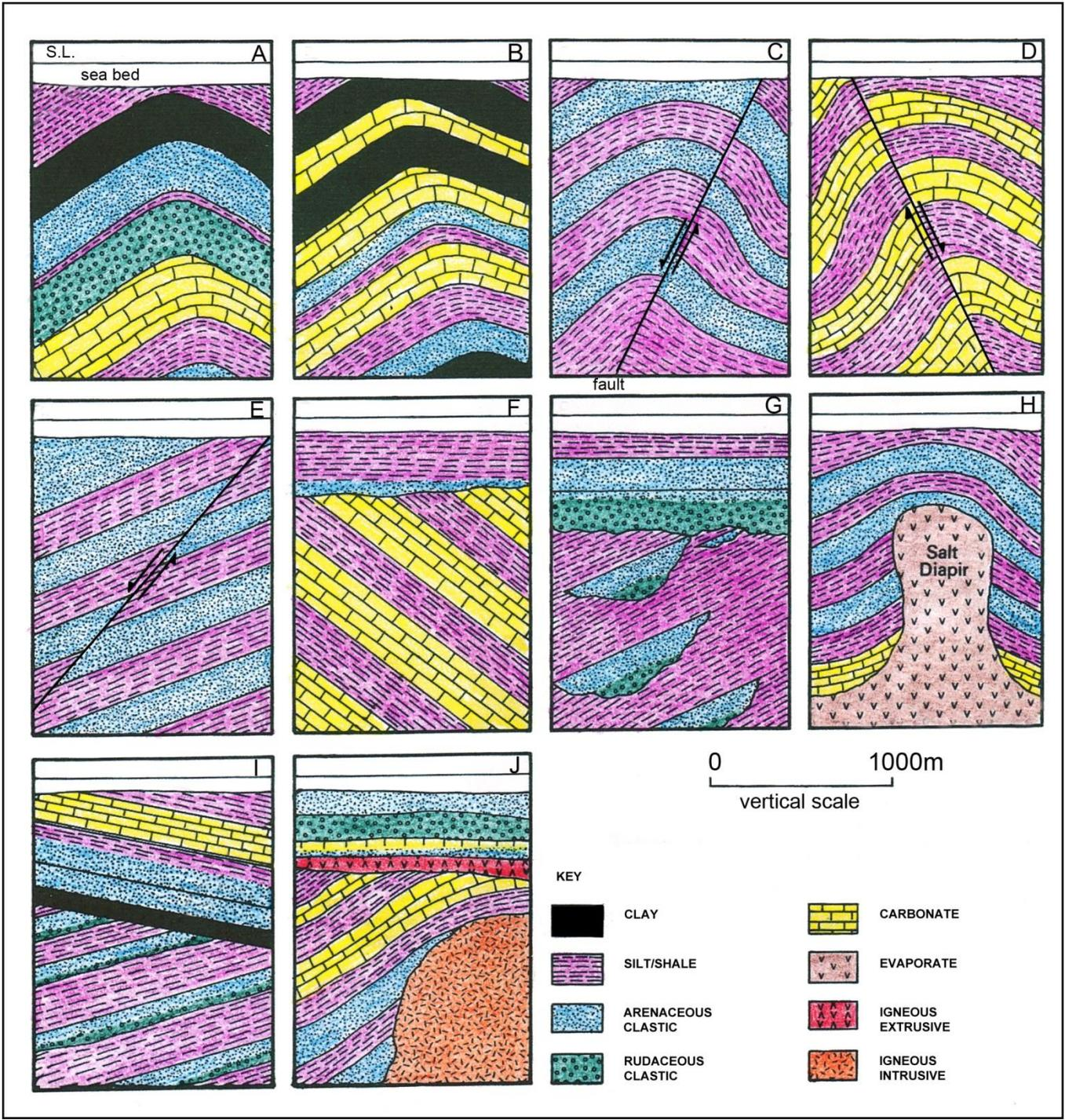
**Figure 4** Section cards showing 10 geological cross sections where there are different lithologies and structures.
